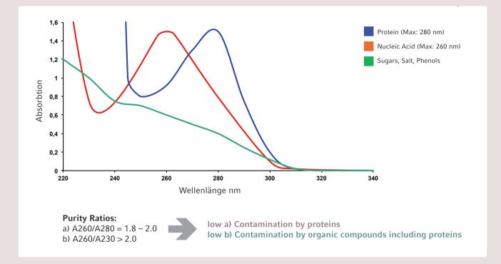
In fig. 8 it is explained how certain types of contamination could influence the measuring result of a nucleic acid sample at 260 nm.
