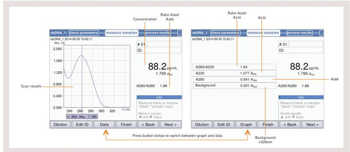
Figure 4: Measuring result of a nucleic acid sample with the BioPhotometer D30 or BioSpectrometer: You can switch between a graphical and table view of the result. In the table view more details about the sample quality is displayed.
