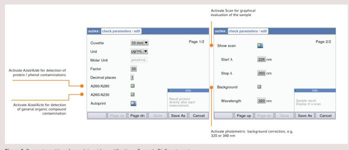
Figure 3: Parameter settings for nucleic acid quantification – Example BioSpectrometer
