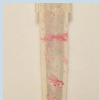
Figure 4: Sample liquid became slightly viscous and had tendency of foam formation after coming into contact with the filter (filter tip from one of the two other manufacturers tested). This observation was made during the investigation, in which distilled water (colorless) was used as test liquid. For visualization, the picture shows test using distilled water with added red dye.
