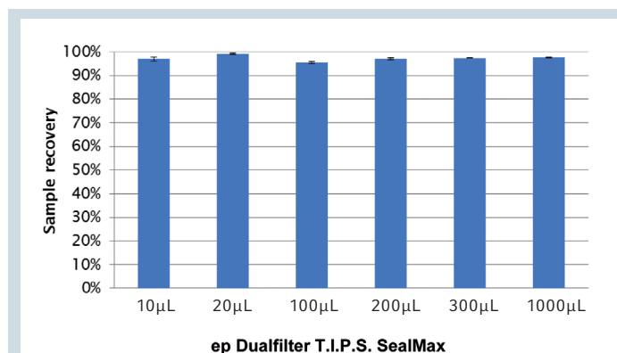
Figure 2: Sample recovery rate of ep Dualfilter T.I.P.S. SealMax following over-pipetting. Values presented are average percentage of sample recovery calculated from 10 individual measurements. The error bar represents standard deviation.
