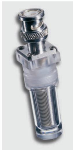
**Fig. 5:** Helix fusion chamber.
