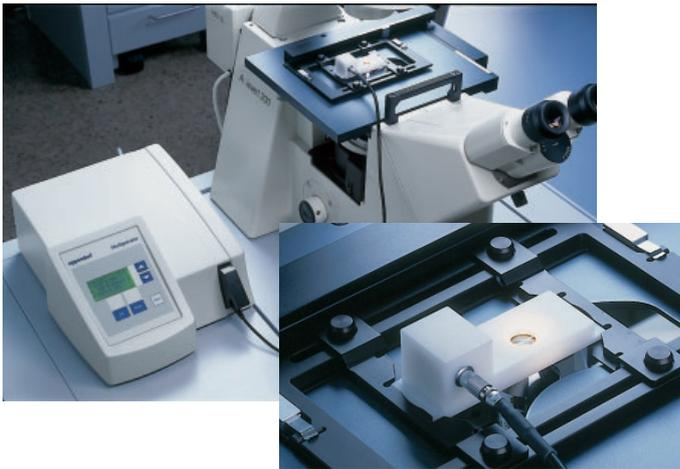
**Fig. 4:** Micro fusion chamber for observing electrofusion under the microscope.
