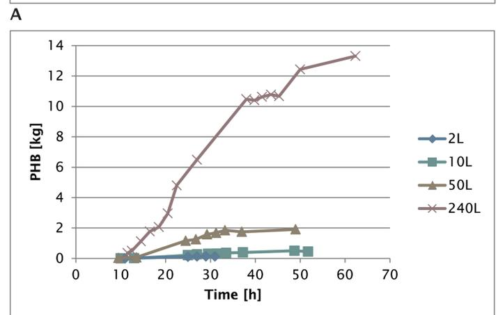
**Figure 4:** Comparison of productivity and total PHB produced in 2 L, 10 L, 50 L, and 240 L fermentation vessels
