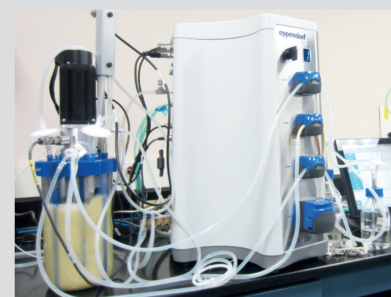
Bioprocess system BioBLU 3f Single-Use Vessel controlled by BioFlo 320 bioprocess control station.
