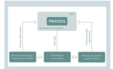
Fig. 1: Ideal configuration in bioprocessing
