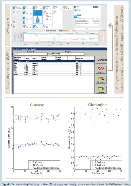
software via OPC. The At-line glucose and glutamine analysis allowed for closed loop control of the nutrients according to the defined set points.
