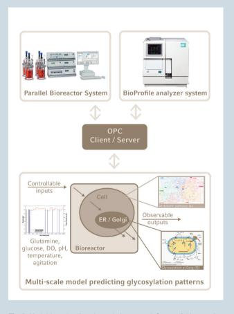
**Fig. 3**: Model-based online glycosylation control. Successful integration of DASGIP Parallel Bioreactors System with a Nova BioProfile 100 Plus analyzer allows for online control of critical cultivation parameters knowing to influence glycosylation (table 1). The multi-scale model utilizes the process variables to predict glycosylation patterns in between actual measurements.
