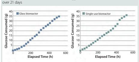
**Figure 4:** Total glucose consumption (Gluc<sub>total</sub>) in glass and single-use bioreactors over 21 days
