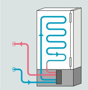
You can improve the conditions and comfort in your lab while saving energy by installing a water-cooled Eppendorf freezer. Many ULT freezers use the air in the laboratory to extract heat energy from the freezer's heat exchanger. Another option is to use a water-cooled ULT freezer connected to a facility's recirculating water system. A constant stream of water removes the heat from the heat exchanger, rather than the ambient air in the lab.
