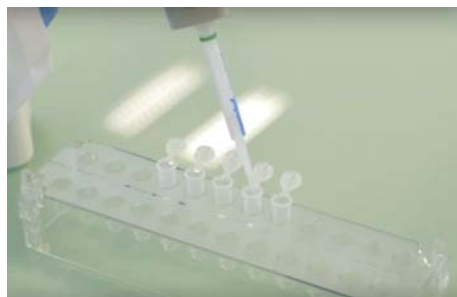
Multi-Dispense the same/different volumes into a set of tubes
