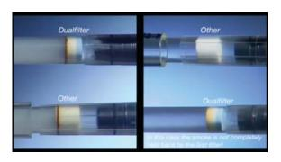
This smoke test show why a dual layer filter from Eppendorf is better than a single layer filter.
