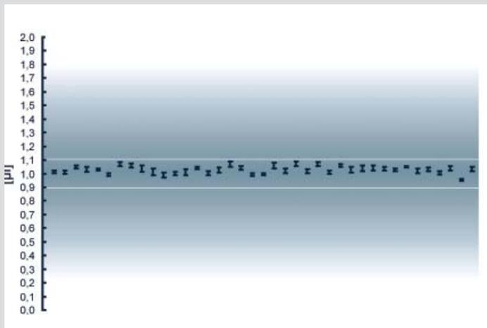
**Fig. 2:** Accuracy and precision of the epMotion single-channel 50 µl tools. Forty tools from different production lots were tested gravimetrically. Each point represents mean value of 10 single measured values for the given tool (in µl) and the error bars represent their precision. Border values for accuracy (+/- 10%) are indicated. Mean value is 1.025 µl. 82% of the tools have the accuracy of +/- 5%.
