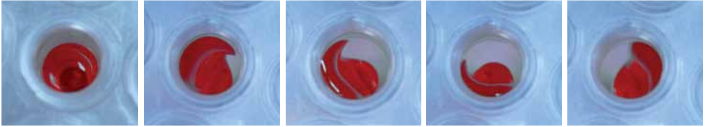
Fig. 1: Time-lapse photography of controlled mixing with the MixMate: One well of a skirted Eppendorf twin.tec® PCR Plate 96 filled with 75 µL water with dye Ponceau 4R is shown without mixing (left photo) and at 1,650 rpm mixing speed (4 time-lapse photos). Due to the 2D Mix-Control technology, the liquid is forced into an orbital flow without chaotic movements, which enables controlled mixing without wetting the lid.
