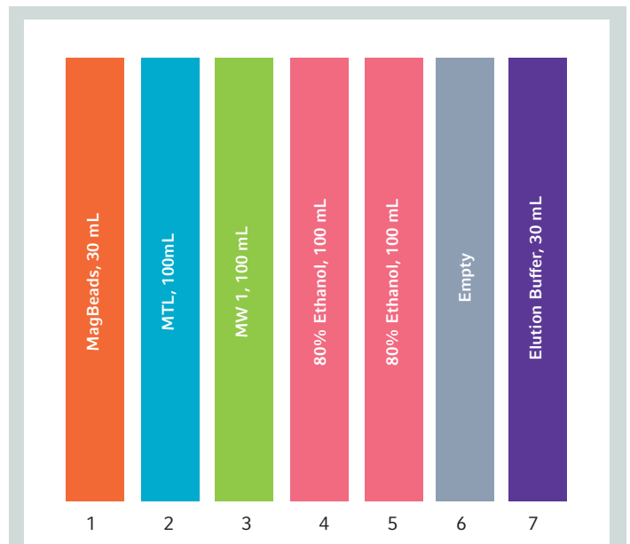
Figure 3: Reservoir rack layout on position C5 of epMotion 5075m worktable. Position 1 and 7 are filled with Reservoir 30 mL. Position 2 to 5 are filled with Reservoir 100 mL.
