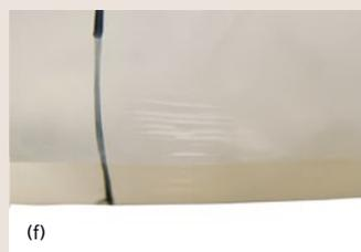
**Figure 1:** Stress lines and bulging (a-f) caused by increased pressure from liquid expansion in 15 mL and 50 mL conical tubes stored in various storage boxes from other manufacturers without temperature compensation vents.
