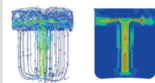
The impeller rotation creates centrifugal force driving medium to circulate uniformly through the entire basket.
