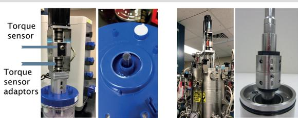
A torque sensor is connected in between the motor and impeller shaft using custom adaptors and bearing modifications. Left: BioBLU 5p Single-Use Vessel. Right: CelliGen 510.
