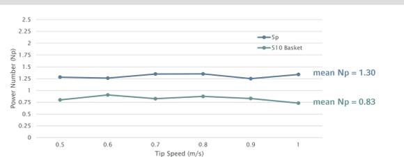
Experimentally derived power numbers for BioBLU 5p and CelliGen 510 packed-bed vessels equipped with cell-lift basket impeller fully loaded with Fibra-Cel.
