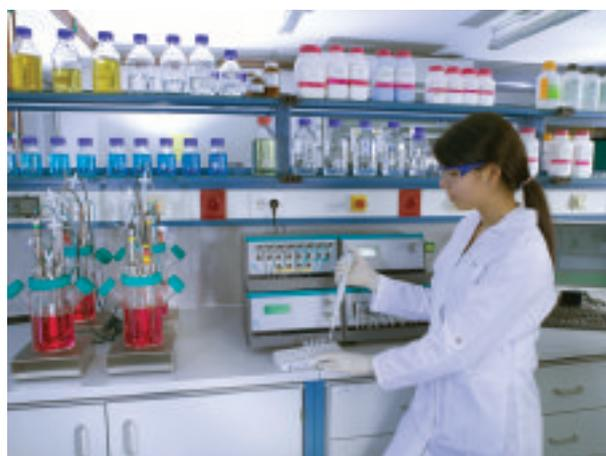
Parallel benchtop bioreactor system for cell culture
