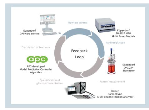
Fig. 2: Integration of external PAT with an Eppendorf DASGIP Parallel Bioreactor System.
