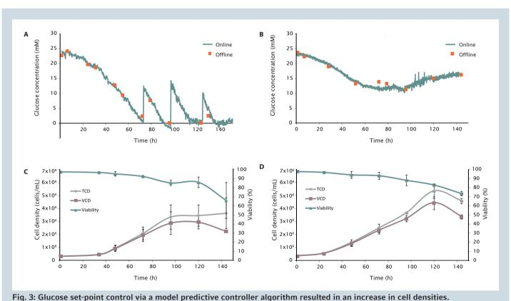
A, B: Glucose concentration was measured online and offline, respectively. (A) Glucose concentration was adjusted via a bolus fed-batch feeding strategy. (B) The glucose set-point was maintained in a continuous feeding fed-batch strategy using MPC.
