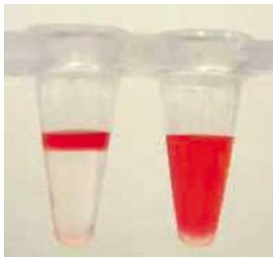
**Figure 1:** Experimental setup before (left) and after (right) mixing with MixMate. Left: Glycerol solutions overlaid with 1/30 volume of red colored water. Right: A completely mixed solution as indicated by the homogeneously red staining without any cords.
