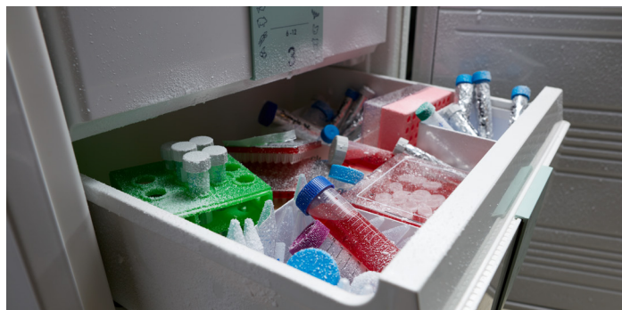
Figure 4: Sample storage without boxes and racks can result in difficulties when samples need to be evacuated
