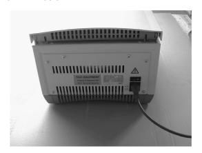
8. Switch on the device at the power supply switch. The lid opens automatically.
