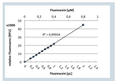
Dosing performance of single-channel 10  $\mu$ L dispensing tool for  $H_2O$  measured by fluorescence spectroscopy (485 nm, 535 nm). Different volumes of 10  $\mu$ M fluorescein in  $H_2O$  were transferred to a final volume of 25  $\mu$ L  $H_2O$ . Standard errors of n=20 repeats are indicated as error bars.
