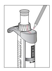
3. Keep the ejector pressed and remove the safety plug with the pin.
