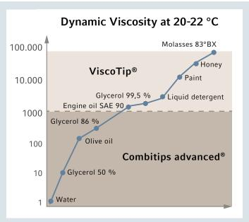
**Figure 2:** Combitips advanced can be used for liquids with a viscosity up to 840 mPa\*s. For liquids with a higher viscosity we recommend using ViscoTip.
