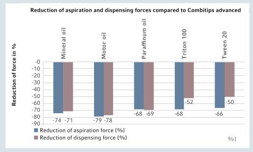
**Figure 1:** Reduction of forces when aspirating/dispensing liquids using ViscoTip compared to Combitips advanced (baseline). n=3
