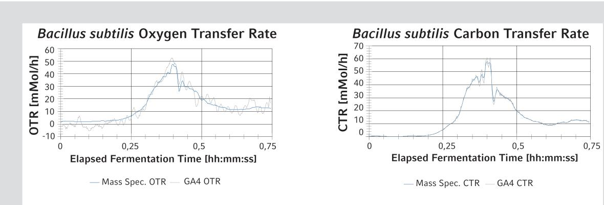
Mass.Spec. OTR recalculated using Fout = Fin \*  $X(N_2in) / X(N_2out)$ GA4 OTR recalculated using smoothed  $XO_2$  signal due to interference with Mass.Spec.
