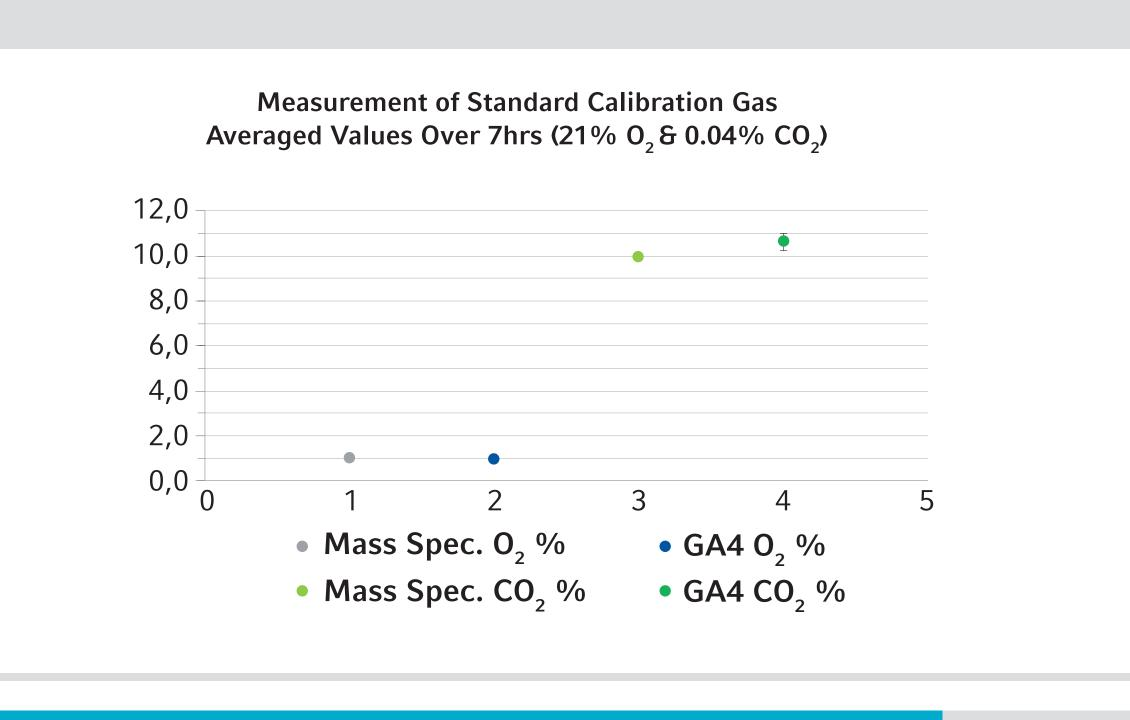
Gas flow measurements from both units demonstrate little interference when two instruments are in the same flow
