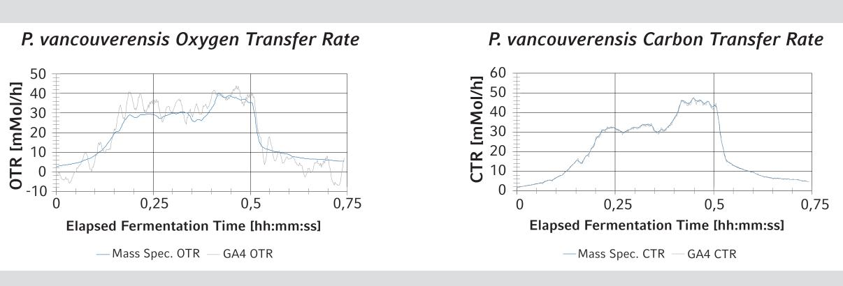
Fermentations of two model strains showed consistent  $O_2$ ,  $CO_2$  and OTR, CTR values ( $< \pm 0.5\%$ ), while also closely matching one another during all phases of growth including lag, exponential, and stationary. In addition, smaller changes in metabolism indicated by changing  $O_2$  and  $CO_2$  evolution were captured by both units.
