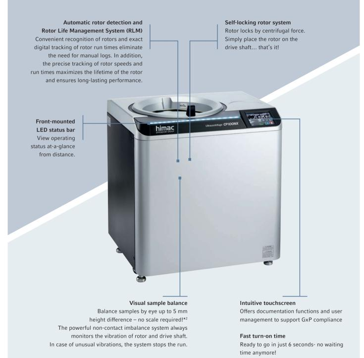
\*1 The CP-NX models are available with max. speeds of 100,000 rpm. For details see last page.
