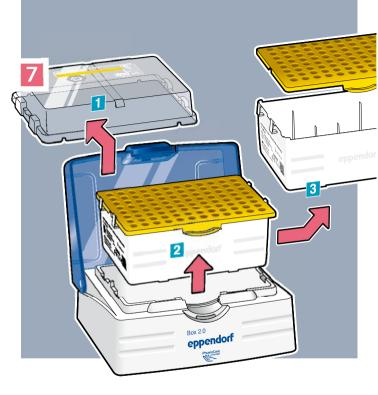
Step 7: Remove the lid 1, then remove the tray and bottom part from the Box 2. Separate the tray from the bottom part 3 for better stackability and to reduce your waste volume.
