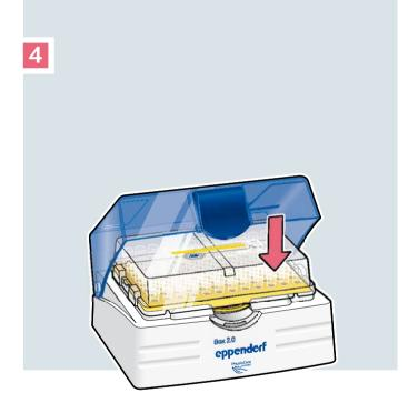
Step 4: Do not remove the lid of the Reload! Firmly close the Box lid over the Reload lid to ensure the TwinLid<sup>®</sup> function.
