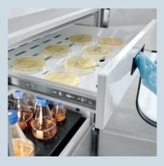
Sample desiccation and medium evaporation protection: The optional culture drawer can be used to protect Agar plates from desiccation. A built-in spill pan and optional humidity monitoring.
