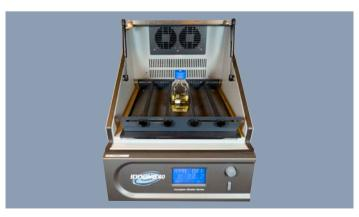
**Optional utility carrier:** Stand-alone platform that quickly fixates vessels between adjustable cushioned rods (no universal platform required, extra rod available)
