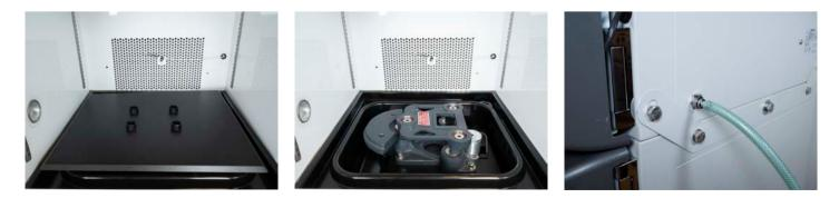
**Spill protected and easy to clean:** The Innova triple-eccentric drive is protected from spills by a covering spill diverter underneath the shaker platform (left). The spill diverter guides liquids to the drainable spill pan with rounded corners underneath (middle and right, tubing and connector not supplied). The built-in spill pan can also be used as water reservoir to reduce medium evaporation – humidity monitoring is optional.
