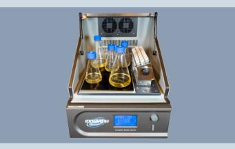
**Flexibility for various vessel formats:** The Innova 40/40R accommodates flasks up to 3L. A sticky pad platform is available for low-speed shaking (200 – 250 rpm, depending on orbit) of flat bottom vessels.
