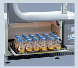
**Easy door and platform handling:** The spacesaving door glides up and out of your way for easy access to all samples and easy service.
