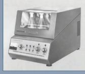
The G-Series, the first incubated shakers, are developed. The triple eccentric drive mechanism is born and is still in use today. For the first time, scientists can grow microbial cultures and solutions under controlled conditions of temperature and high rates of agitation.
