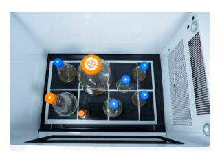
**Flexibility for various vessel formats:** The Innova 43/43R accommodates flasks up to 6 L. A sticky pad platform is available for low-speed shaking (200 – 250 rpm, depending on orbit) of flat bottom vessels.
