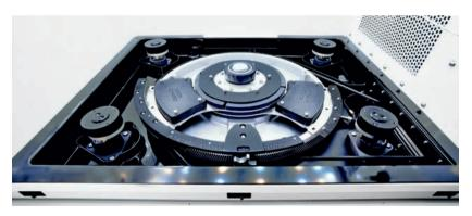
Built to perform and last – the patented Eppendorf X-Drive: With it's five eccentric mounting points for the shaker platform, the drive is precisely engineered to ensure long-lasting, repeatable performance with high loads over years. The four shafts in the corners and Balance Master Technology support precise vibration-free shaking on every point of the platform, including the periphery.
