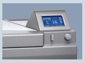
**Easy interface handling and programming:** The top-mounted controls and display make it easy to view, set and program parameters - continuous, timed, or multi-step programs with up to 15 steps (four programs storable).
