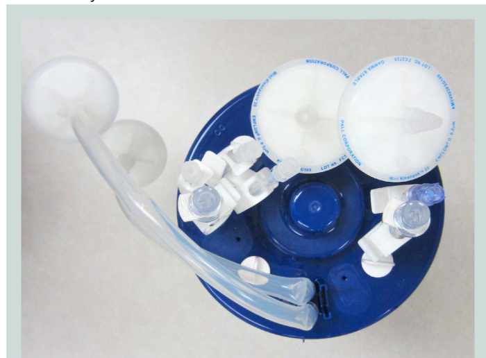
Fig. 2: The head plate of a BioBLU 3f Single-Use Fermenter.
