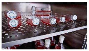
Removable shelf enables shaking of suspension cell cultures while incubating adherent cells under the same conditions
