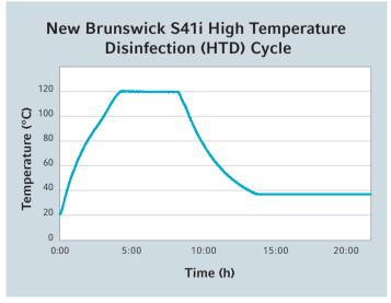
The HTD feature heats the internal chamber to 120 °C and holds it for 4 hours to effectively eliminate contaminants
