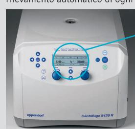
Error 15 Imbalance Load rotor symmetr., check load ever Press OPEN, repeat run. 30:00 min 2410 rcf
