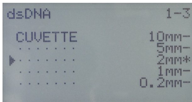
Fig. 2: Programming of the 2 mm light path in parameters for the method dsDNA
