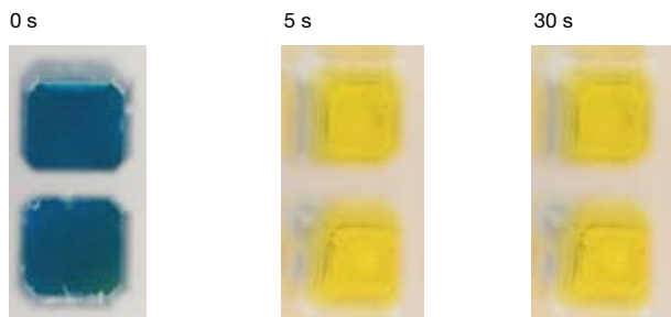
Fig. 2: Resuspension of sucrose pellets with bromothymol indicator solution in an Eppendorf Plate Deepwell 384/200 \mu l and in two corresponding deepwell plates from other suppliers. The plates were mixed immediately after the addition of the indicator solution (0 s) in the MixMate at 2000 rpm and photographed after 5 s and 30 s
