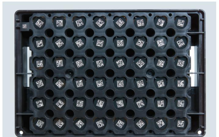
With the Eppendorf RackScan and software, you can scan more than one vial in parallel and transfer the sample data to your sample management software, e.g. eLABInventory or external databases
