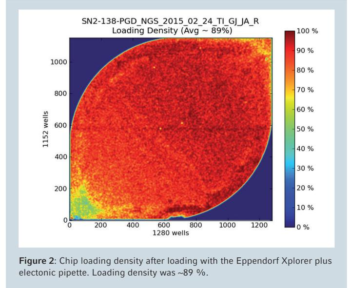
Another parameter relevant to the method's evaluation is the reproducibility of the loading level. During the operators' manual pipette handling, the coefficient of variability was reaching more than 24 %, making it difficult to ensure efficient loading level in every run. Switching to the electronic
