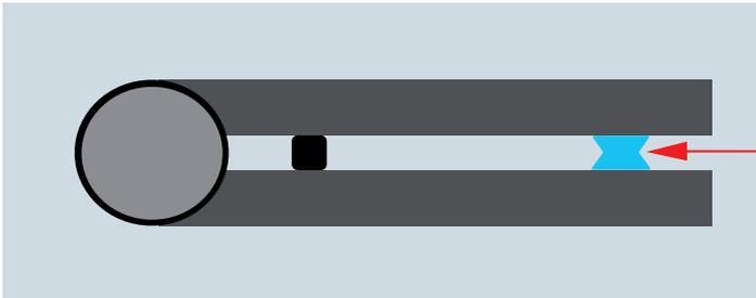
**Fig. 5: Diagram of the  $\mu$ Cuvette.**
