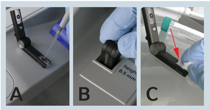
**Figure 6: Measurement process with the  $\mu$ Cuvette:**
