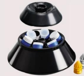
Centrifugation up to 17,000 × g \* with rotors for 50 mL conical tubes, e.g. 59xx series and 58xx series:
