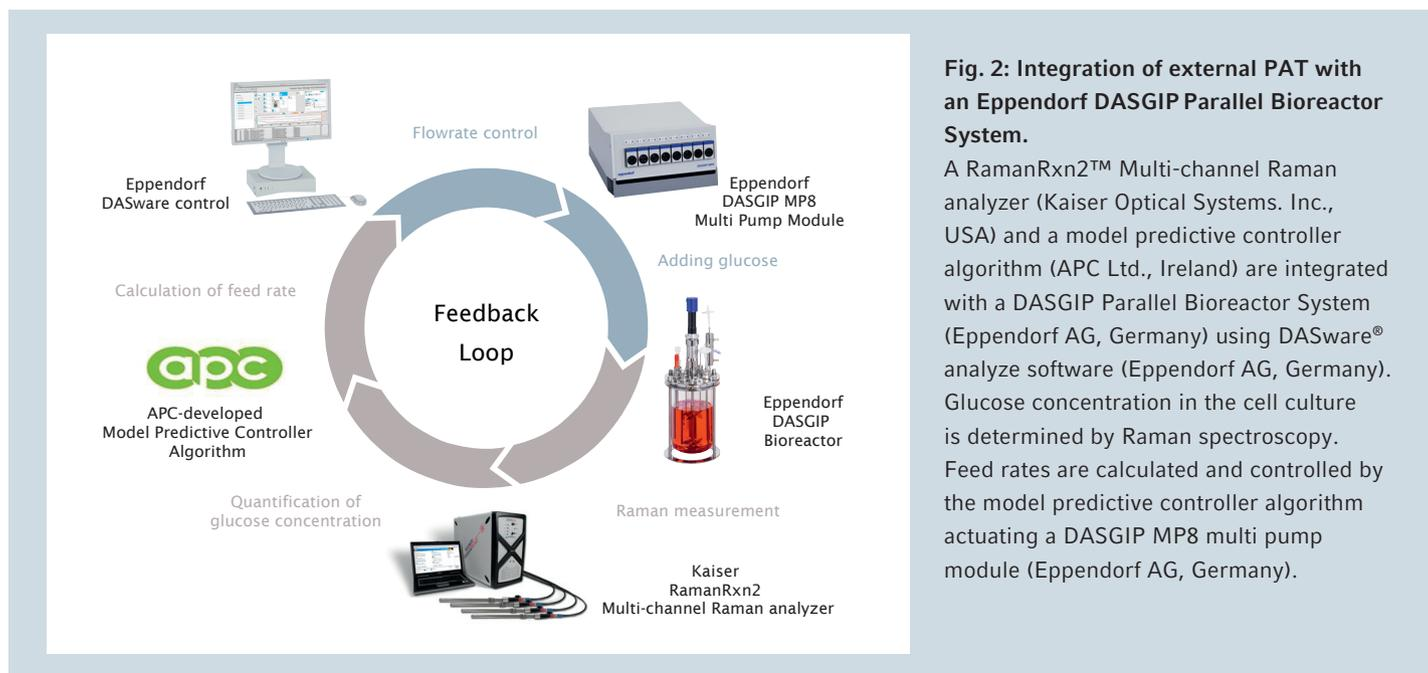
**Fig. 2: Integration of external PAT with an Eppendorf DASGIP Parallel Bioreactor System.**
