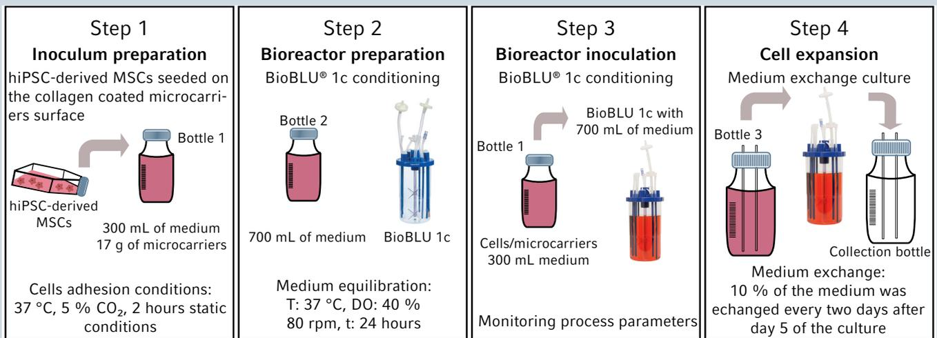
Fig 3: Process flow diagram of the experimental setup
