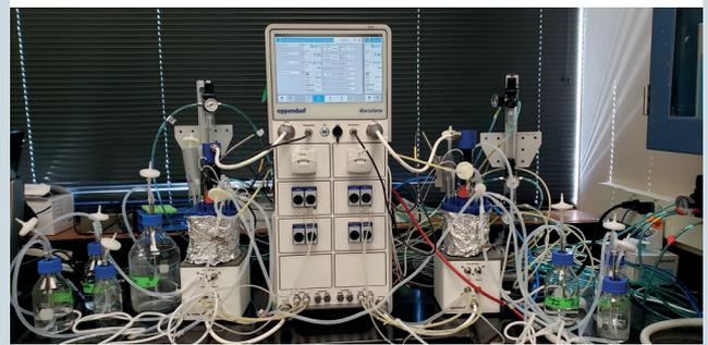
**Fig. 1:** Human iPSC-derived MSC exosome production in a medium exchange-batch culture using the SciVario twin bioreactor control system and BioBLU 1c Single-Use Bioreactors.
