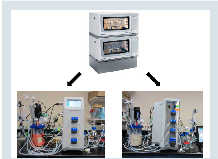
Fig. 3: Key equipment used in this Pichia pastoris fermentation and protein production workflow.
