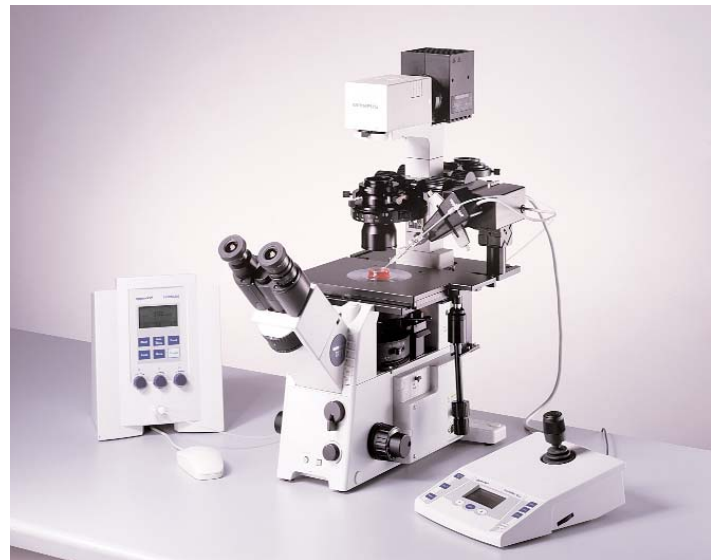
Fig. 1: Workstation for semiautomatic microinjection into adherent cells: Olympus microscope with Eppendorf InjectMan NI 2 and microinjector FemtoJet
