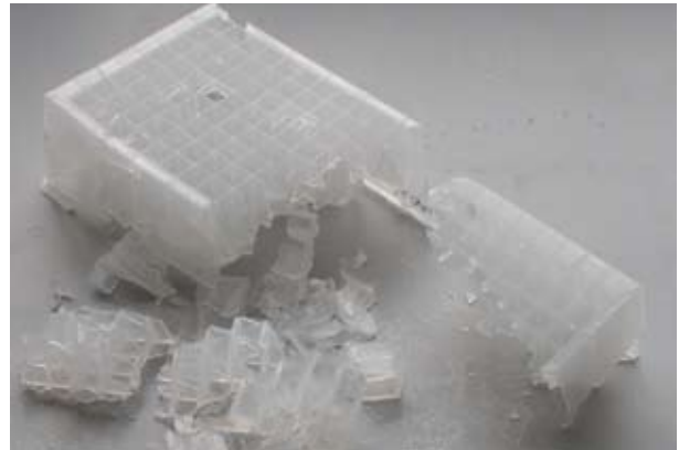
Fig. 2: Fragmented competitor's plate following centrifugation with 70 % ethanol (4 °C, 90 min) at 6,189 x g in the Centrifuge Sigma 4K15C, Rotor 09100.
