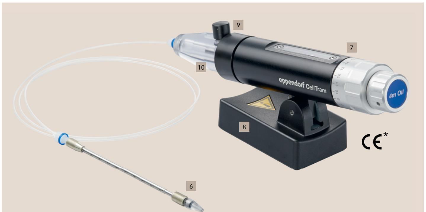
6 New grip head 4 system for simple capillary change and higher user safety
