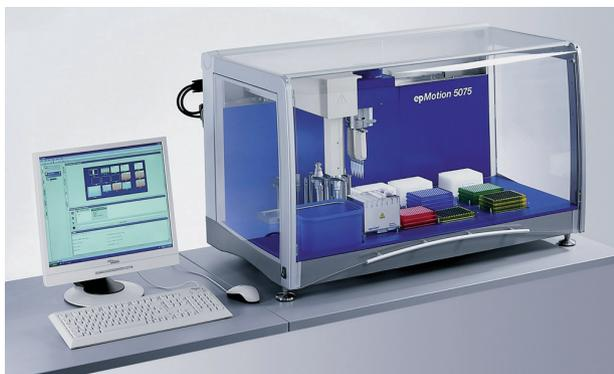
Figure 1: epMotion 5075 LH, Version with PC software
