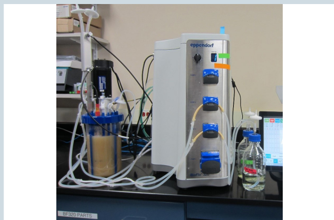
Fig. 5. Lactobacillus acidophilus fermentation in the BioBLU 3f Single-Use Vessel controlled by BioFlo 320.
