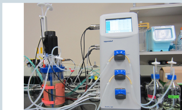
Fig. 3. Lactobacillus acidophilus fermentation in the BioBLU 3f Single-Use Vessel controlled by BioFlo 120.
