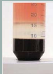
Gradient formation of blood sample with Centrifuge 5702's SOFT function
