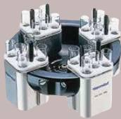
Swing-bucket rotor for 24 x 15 mL glass tubes
