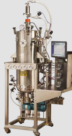
BioFlo 610 Pilot-scale SIP fermentor 13 - 100 L working volume
