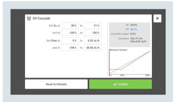
Fig. 2: VisioNize-onboard user interface - DO cascade screen
