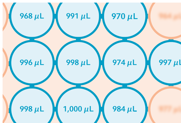
10 measurements – avg. 984 µL, 1.6% error
