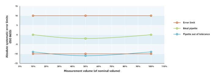
ISO 8655 requires three volumes to be tested during calibration: Nominal volume, 50% of nominal volume, and the lower limit of usable volume or 10% of nominal volume (whichever is greater). Since the error limits of a pipette are not linear from the minimum to maximum volumes, it is possible that the 10% and 100% volumes perform within the systematic error limits while the 50% volume does not.
