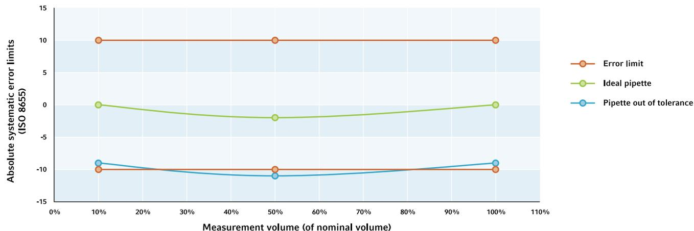
ISO 8655 requires three volumes to be tested during calibration: Nominal volume, 50% of nominal volume, and the lower limit of usable volume or 10% of nominal volume (whichever is greater). Since the error limits of a pipette are not linear from the minimum to maximum volumes, it is possible that the 10% and 100% volumes perform within the systematic error limits while the 50% volume does not.
